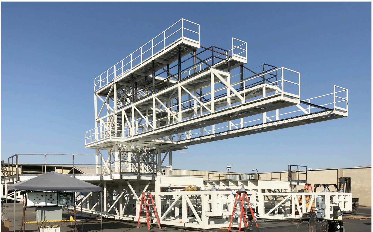
30 feet tall, 50,000 pounds Kern Steel Multi-Level, Multi-Aircraft Maintenance System powered by Duff Norton Automated Actuator System (AAS) controls.
